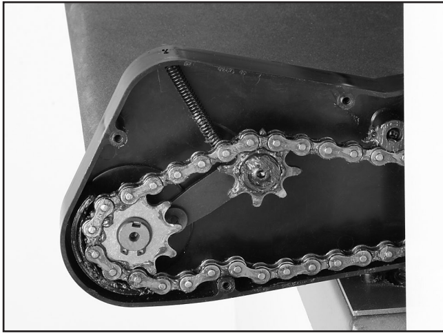
Figure 28. Feed belt drive chain.
